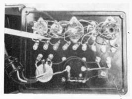
Fig. 9: Back view of the front panel. The resistor's shown protect a DM70 from overload during test."
