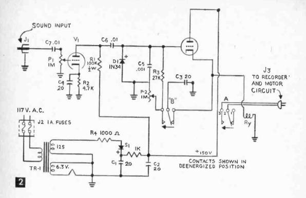
potentiometer P1 is fully clockwise. The motor will run continuously as long as loud enough sound is fed continuously into the microphone as in normal operation. This will happen under the conditions mentioned regardless of the setting of delay control, P2.
