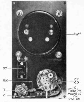
FIG. 3: During the early stages of construction, we see the resistors, R1 through R9, mounted on the terminals of the switch.
