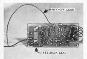
Fig. 5: Adding the pick-off lead and the feedback lead. Dress the feedback lead close to the chassis.
