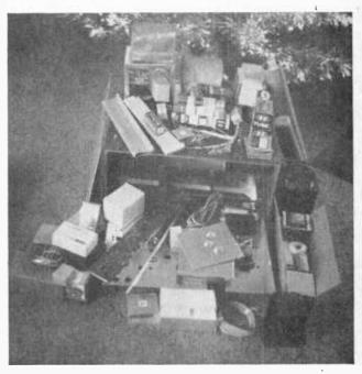
FIG. 1: Resistors, capacitors, tubes, coils, crystals and other things the builder probably won't even recognize until construction begins.
