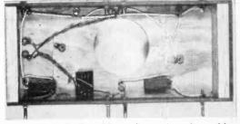
Fig. 11: Underside of basic chassis shows how wiring is dressed around center hole and filament leads are twisted for anti-hum.
