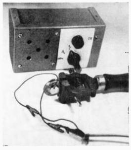
You can use the Amplagimik for testing microphones. Lock the microphone in a vise and measure output.
