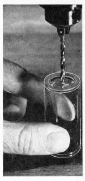
FIG. 2: First, drill three small holes in the bottom of the vial. The one in the center should be the same diameter as your stove bolt. The other two are drilled close to the edge of the bottle on opposite sides, large enough for lead wires on the capacitor.
