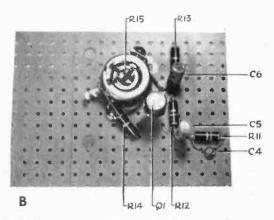
FIG. 4A, 4B: The mounting board, front and rear views. Notice the 1/8-in. holes for feedback control.
