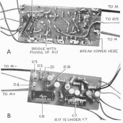
FIG. 5A, 5B: Modifications to the amplifier unit.
