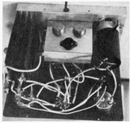
The filter installed in a battery eliminator.
