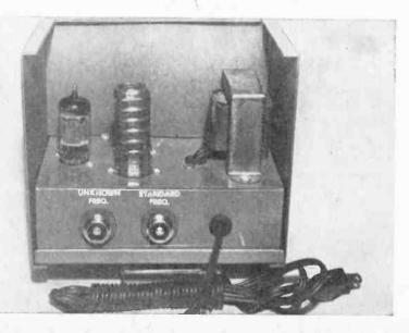
FIG. 4: Microphone connectors are shown for input and output terminals. Use any coaxial connec-
