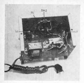
Fig. 8: On top of the chassis, we see the positions of the tube, relay, transformer and locations of the controls.
