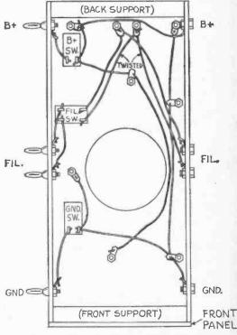
FIGURE 5: PICTORIAL WIRING
