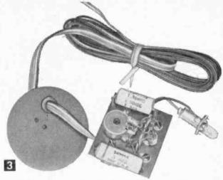
Circuit wiring can be done in about three hours. Parts mount on a plastic chassis which fastens to the back of the meter dial.
