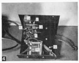
Fig. 4: Underneath the chassis inside the finished sound relay. Dress diode D1 to avoid short circuits.
