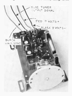
Fig. 1: The Lafayette PK-633 subminiature AM broadcast tuner is the heart of the unit. You only need box and phones.
