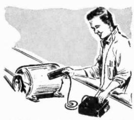
An electric motor generates a spark, which is in essence, a radio signal. The pickup acts as a probe permitting you to hear the sound of the motor. In a short time, you learn the sound of a healthy motor, and after some practice, can even detect symptoms!
