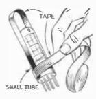
cured around the bottom with another strip of tape. Don't use tape on tubes that heat up excessively, because of the possible danger of fire due to tape igniting. *Never* use plastic tape for this purpose as it ignites easily.
