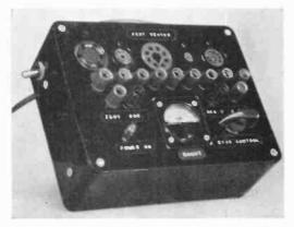
Fig. 2: The PERT tester uses 13 binding posts and five tube sockets to program test electron ray tubes.
