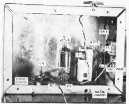
Fig. 4: With the cover removed, we see the location of the major components. Note capacitor C1 protruding.
