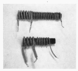
Fig. 4: The coils, wound on ferrite with insuloted wire.
