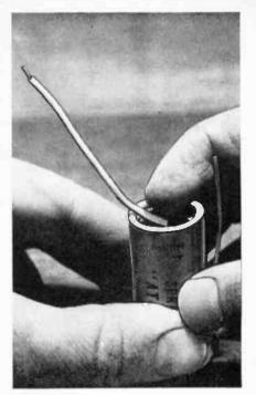
FIG. 3: Dress negative lead wire of capacitor closely up the side of capacitor, toward positive end. Put a sleeving on the positive lead. If you have no sleeving, slide the insulation from a piece of bell wire and use it. Cover positive end of capacitor with friction tape. Install the stove bolt in the vial with the head inside the bottle.
