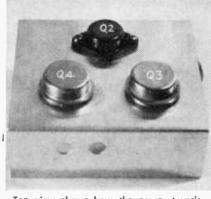
Top view shows how the power transistors, Q2, Q3, and Q4 are mounted. No extra controls are required in normal use.
