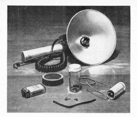
FIG. 1: Items in foreground are all that are needed to convert the flashgun into a more dependable, economical B-C unit; 22.5-volt "B" battery, small piece of friction tape, plastic pill bottle, rubber bands, 250 mfd 25-volt capacitor, small bolt, two nuts, and sleeving.
