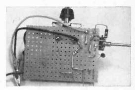
Fig. 3: The under-chassis view shows the clip leads for coil connections. Using clip leads facilitates coil changing.
