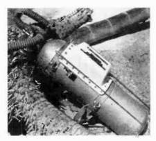
The product on model in position on a scuba tank. The on-off switch is at the bottom. Future models will have even more compact antennae. Units also carry lights which indicate if batteries have full charge.
