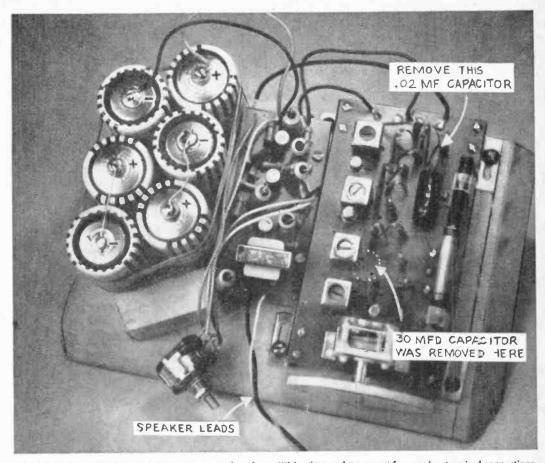
FIG. 5: Batteries, amplifier, and tuner are mounted on base. Wiring is complete except for speaker terminal connections.
