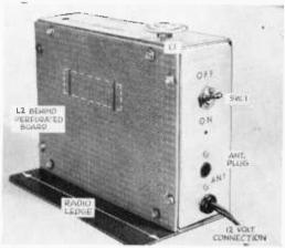
Fig. 5: The side view shows the on-off switch and the antenna jack. The line cord connects to the battery.
