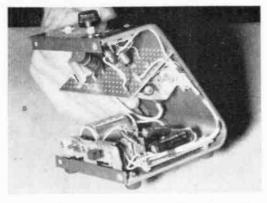
FIG. 5: Inside the unit from the rear. Note the mounting of the dry rectifier and the capacitors in the filter system.
