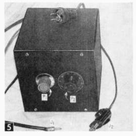
Fig. 5: Front view of the completed unit. Only two wires are used, one for signal and one for power. P1 controls the sensitivity of the unit, P2 the time delay.
