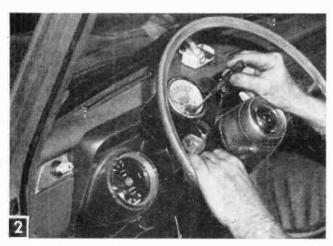
Space between the dash and steering column on this import car was limited. But a good fit was made by mounting the housing casting backwards. Eit brackets also make over or under-dash mounting possible.
