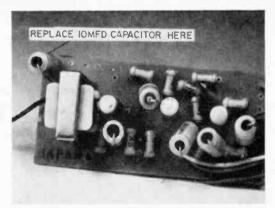
Fig. 5A: Top view of amplifier board after modification. The 10 microfarad capacitor is soldered into position.
