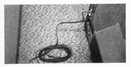
FIG. 8: It may seem wasteful to cut all that lovely twinlead, but that coil behind the TV set is robbing your signal.
