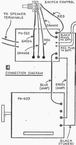
REMOVE ALL TUNER LEADS EXCEPT BLACK (RIGHT ABOVE) AND MAKE CONNECTIONS AS SHOWN
