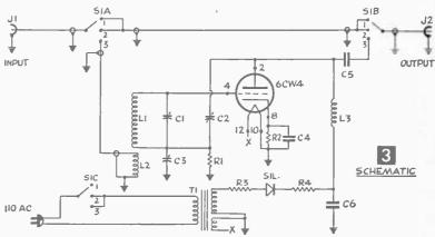
transformer. Mount input and output connectors on the rear panel. The remaining components are dish-mounted on a 5x2% in. Ushaped chassis of 16 in. aluminum which is secured to the front panel with 6-32 screws. Insert the 6CW4 tube in its socket between the chassis and the front panel. Mate the shaft of C1 to the insulated coupling of the dial. Figure 2 illustrates rear panel construction of the finished amplifier.
