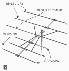
FIG. 3: The open end of the double vee should face toward the transmitting station, like the open mouth of a funnel.
