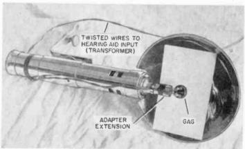
FIG. 3: You can mount a microphone facing into any parabolic reflector, such as a flash gun. Also lamp shades, or auto headlamp reflectors from old cars. Result is a very highly directional effect for long distance use.
