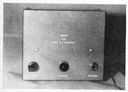
FIG. 1: The front panel for the mixer is finished with decals for a professional appearance. Use care during drilling, punching, to avoid scratches.
