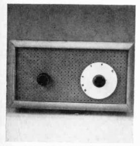
FIG. 8: Front view of completed receiver. Left knob controls power on-off and volume. Right knob controls station selector.
