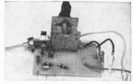
Fig. 2: Top view of the tuner. Note that the potentiometer is supported to the mounting board only by its connections.
