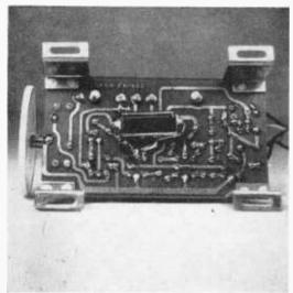
FIG. 2: Remove the 30 mfd. AVC bypass capacitor shown here and replace with a 2 mfd. capacitor for better fidelity.
