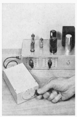
Fig. 3: Shown here with an amplifier, the unit delivers AM radio reception. Note the home-made vernier tuning device.
