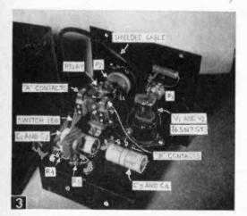
Fig. 3: Parts location on top of the chassis of the completed unit. All controls mount on front panel.
