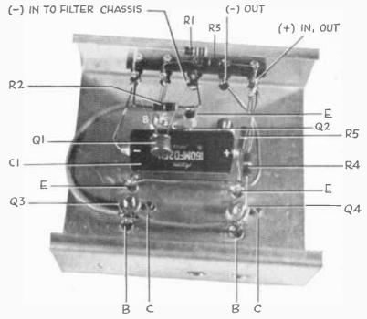
Looking at the bottom of the wired chassis, the locations of the various components is clearly seen. Notice the long transistor leads and the wide spacing of components to permit easier and more rapid cooling below the main deck.
