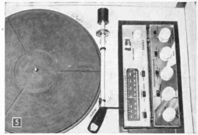
Turntable, transistorized Knight-Kit stereo FM tuner, and 40-watt amplifier fit in center section. Chassis rest on cabinet bottom; are framed with quarter round.
