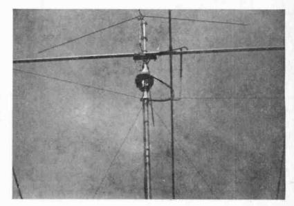
FIG. 4: An antenna rotator is controlled from inside the house and permits you to point the antenna where it's needed.
