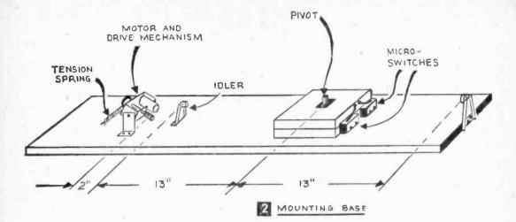
these are attached, drill a \(^3\)e-in. center hole and a \(^1\)e-in. id flanged threaded bushing (1 in. or longer) and install it from the bottom with a large washer under the flange and fastening nut. Drill a \(^3\)e-in. hole into the center of the cross pieces and chip out the bottom to provide clearance for the washer and nut. Force fit the cross pieces over the bushing and nail or screw into place. To obtain extra support, two idler wheels are
