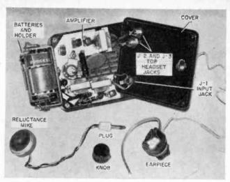
FIG. 6: The parts placement is easy to see. When the amplifier is completely installed, the cover fits over the case so the volume control shaft is run through its matching hole. Then replace the knob.
