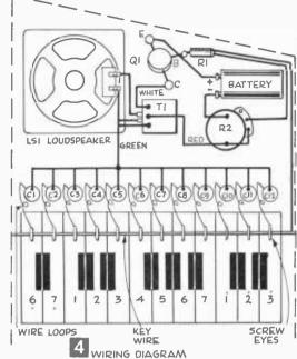
thumbtacks. Potentiometer R2 requires a hole for its shaft. The battery and transformer T1 are held in place with conventional brackets. If the piano has a one piece top, it will be necessary to cut holes for the loudspeaker. With a hinged top, the loudspeaker should be tilted.
