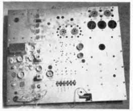
FIG. 3: Above, This is the wired chassis base assembly. The arrow shows the two backward mounted diodes, the only confusion resulting in error in construction.
