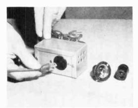
FIG: 7. The plug on the cord from the hearing aid to the supply is widened by soldering a piece of brass to one leg. This prevents you from connecting to a live outlet.
