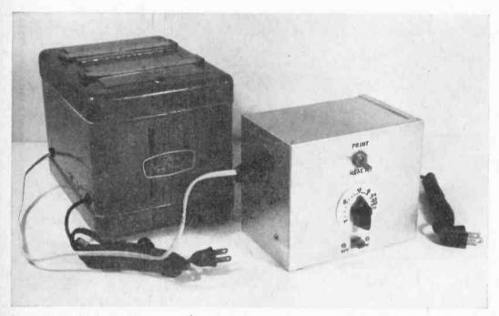
Fig. 9; The completed unit with a contact printer plugged in. Notice the white plastic dial scale that you calibrate.
