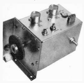
FIG. 5: The VFO is built as a separate unit and then mounted on chassis top plate. It is temperature compensated and always stays "on" regardless of position of function switch. VFO draws only 4 watts.
