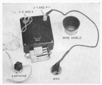
FIG. 4: Mount the microphone unit to a surplus telephone shield, and plug in. While the directional effects are not as good over great distances as the reflector, side noise is cut down considerably.
