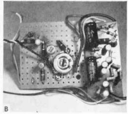
FIG. 7 A-B: Top and bottom views of circuit board with amplifier unit in place after modification.
