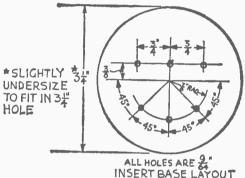
FIGURE 7: POWER TRANSISTOR INSERT
