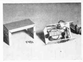
FIG. 6: Looking into the power supply box we see the transformer, line fuse and the modified receptacle.
