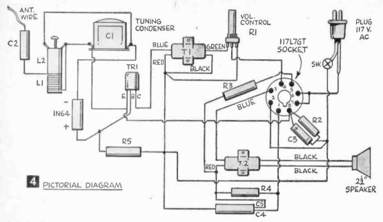
heard. If not, check the voltage from pin 1 of the rectifier section. About 120 volts should be noted at this point. Check the voltage on the plate of the output tube. The trouble can be found by using the voltage and resistance check method. If a hum is heard on pin 4 proceed to the base of the transistor. A louder hum will be heard if working properly. The volume control must be full on. A positive 4½ volts will be found on the emitter
