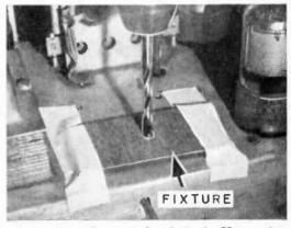
where the hole is to be drilled. Using this drilling fixture, there's no need for a center-punched indentation to start the drill.—J.A.C.
