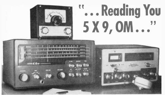
FIG. 1. This preselector will add 20 db of signal at 28 mc, and nearly 30 db at 14 mc. It's a must for the HAM or SWL with a lower-cost receiver!
