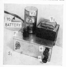
Fig. 1: All parts mount on a small open-end chassis with the on-off switch and the output on one side.
