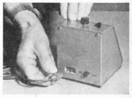
FIG. 3: A recessed TV plug connects the unit to the power supply. The slide switch permits the user to select modes. You can choose at line operation by sliding the switch right, or battery (built-in) by sliding switch left.
