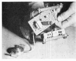
FIG. 8: With the case opened and the chassis removed, we see parts on the perforated Bakelite board. Note that all parts mount on case to facilitate opening.
