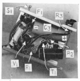
Fig. 2: The under chassis view shows the location of all parts. Be careful to observe proper polarity on the electrolytic capacitors and diodes to avoid damage.
