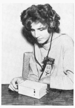
Fig. 2: The unit can be used either with earphones directly, or with any amplifier to drive a good-sized loudspeaker system.
