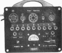
for Programmed Electron Ray Tube. Fiveway binding post terminations for all tube socket and built-in power connections, allow a circuit to be "programmed" with jumpers and external resistors or capacitors.
