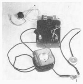
FIG. 5: Connect a plug to one end of a 25-ft. length of phono card and a plug to the other end. Keep the spool with your amplifier for use when long runs are needed between the mike and amplifier units.
