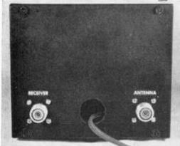
FIG. 5. The rear view shows the power cord and the two coaxial connectors. One goes to the antenna, the other to the receiver.
