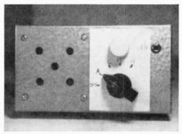
Fig. 10: Make up the switch plate from a piece of card. You can type or hand letter the information. Paste the card down to the panel with rubber cement.
