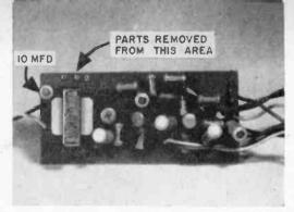
Fig. 4: Modify the circuit board on the amplifier. Carefully remove the unused components (See text).
