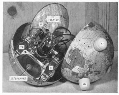
The radio is built on a plastic sheet which, when complete, fits into a dime-store globe.
