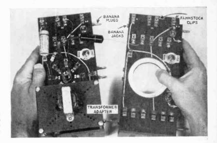
Fig. 8: With one stage complete on the left chassis, a second chassis is plugged in for development of next stage.
