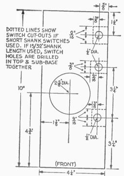
ALL OTHER HOLES IN TOP & SUB-BASE TOGETHER FIGURE 2: PLYWOOD SUB-BASE
