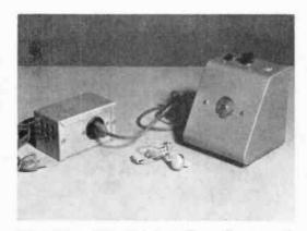
FIG. 2: The complete equipment. The small power pack can be placed on the floor near an outlet. A built-in battery pack permits the user to disconnect from the supply. While not miniature, it is portable on batteries.
