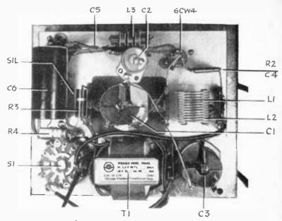
FIG. 2: Looking inside the preselector, you see placement of component parts.
