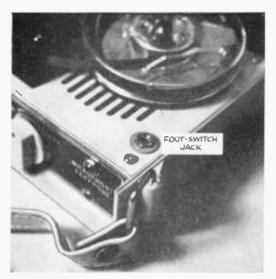
FIG. 1: Locate the jack for the foot switch on the front panel. Place it so the foot switch cord will not interfere with normal tape recorder operation.
