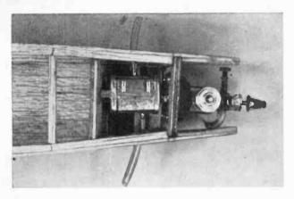
FIG. 3: Engine overflow and filler tubes extend out through sides of fuselage. Gas feed line comes under engine and connects to right side at fuel intake nipple.
