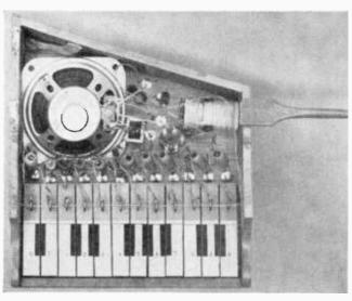
FIG. 1. With the lid removed, the wiring is clearly seen. Notice that the wire loops between the keys and the capacitors provide additional flexibility and prevent the wire from breaking under use.
